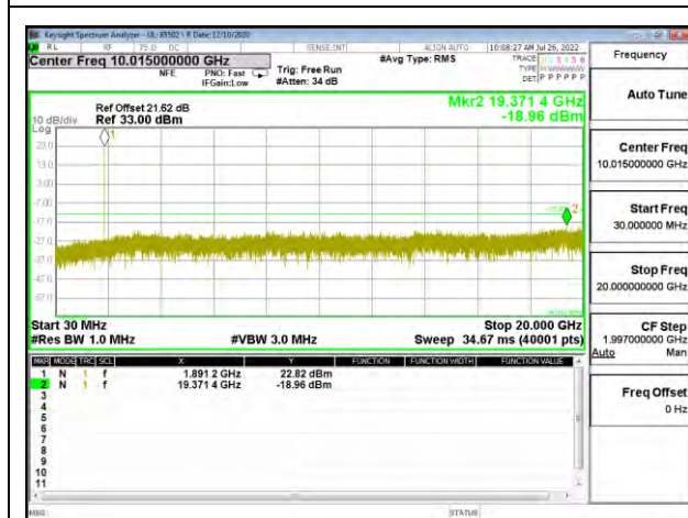
LTE2 20MHz QPSK HIGH Ch RB1-0
