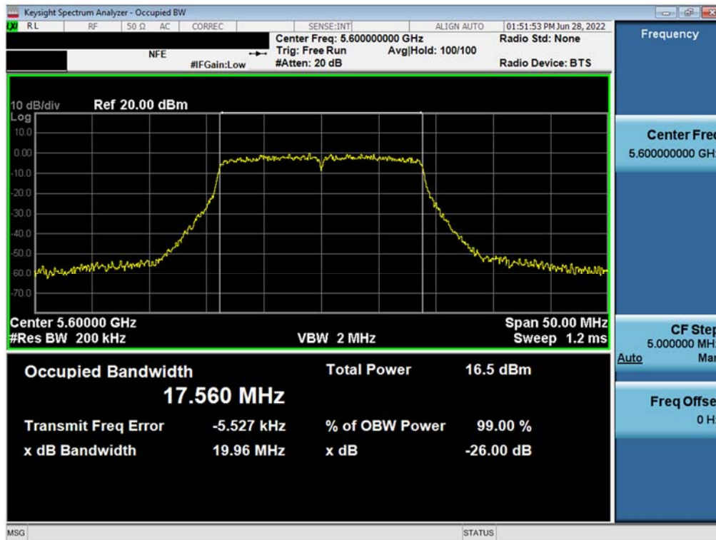
Plot 7-92. 26dB Bandwidth Plot MIMO ANT2 (802.11n – 20MHz BW (UNII Band 2C) – Ch. 120)
