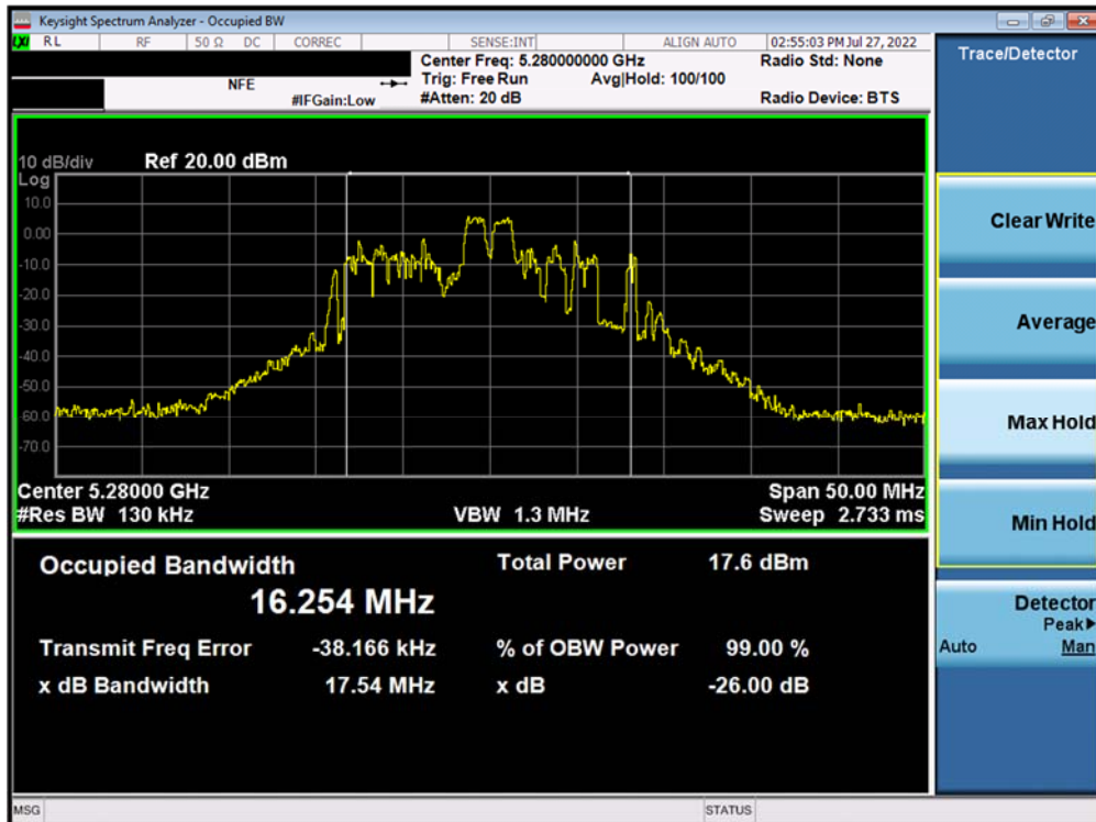
Plot 7-58. 26dB Bandwidth Plot MIMO ANT2 (20MHz BW 802.11ax – 26 Tones (UNII Band 2A) – Ch. 56)
