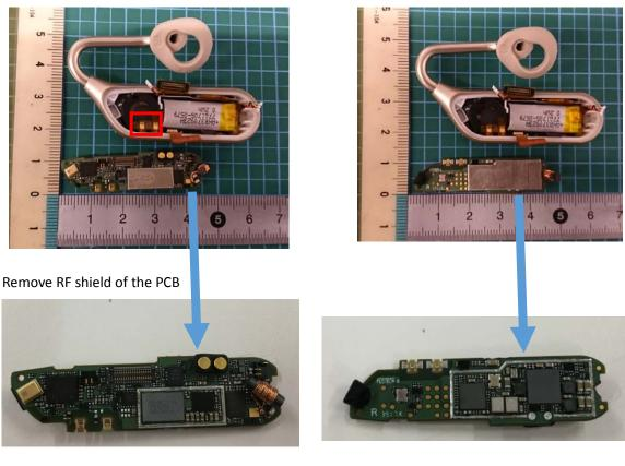
Remove battery (battery front and back)
