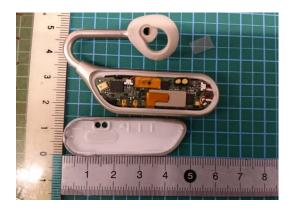
Remove PCB (below RED box is the antenna location for bluetooth)
