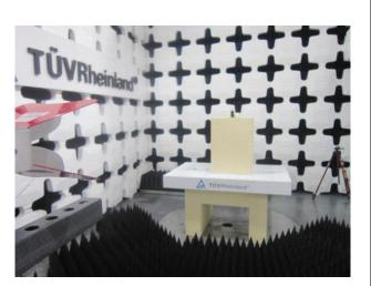
RADIATED TEST SETUP
