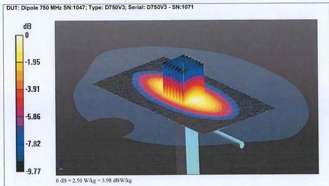
Communication System: UID 0, CW; Frequency: 750 MHz; Duty Cycle: 1:1 Medium: 750,835,900,1800,1900 MHz HSL Medium parameters used: f = 750 MHz;  $\sigma = 0.914$  S/m;  $\epsilon_r = 41.936$ ;  $\rho = 1000$  kg/m<sup>3</sup> Phantom section: Flat Section DASY5 Configuration:
