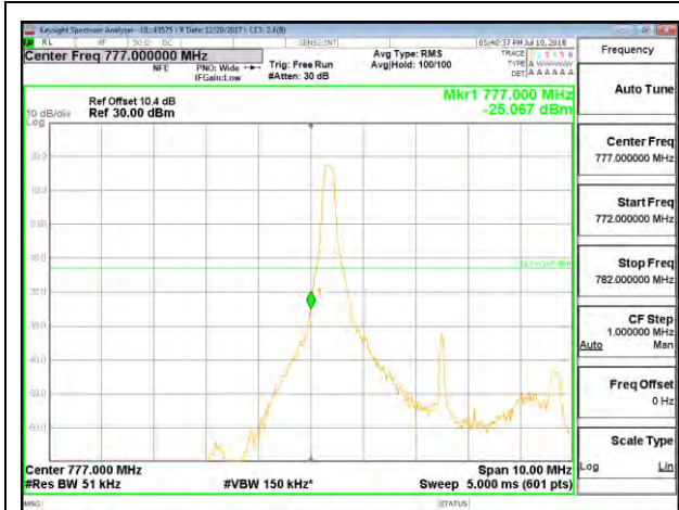
LTE B13 5MHz QPSK Low Channel RB1-0
