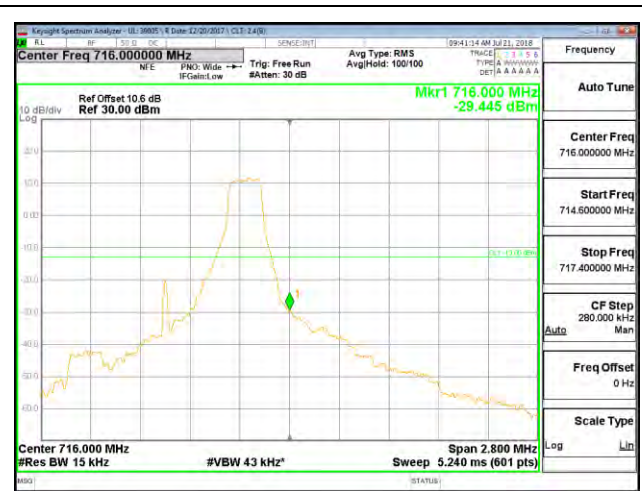
LTE B12 1.4MHz 16QAM High Channel RB1-0
