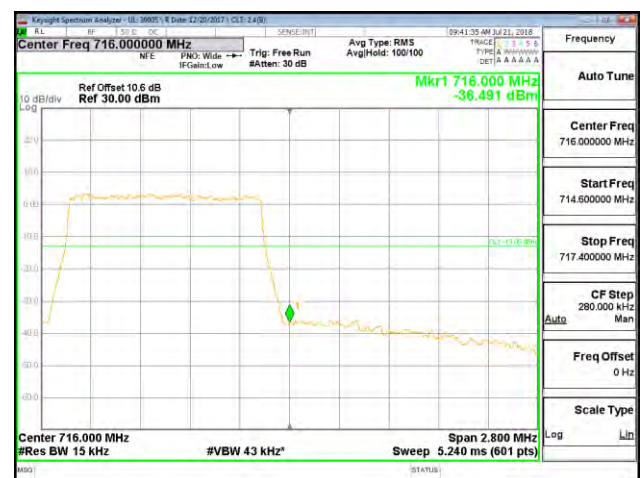
LTE B12 1.4MHz 16QAM High Channel RB6-0
