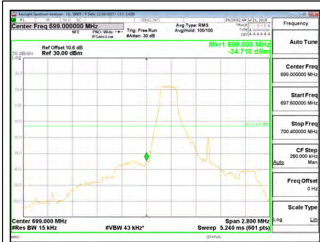
LTE B12 1.4MHz QPSK Low Channel RB1-0
