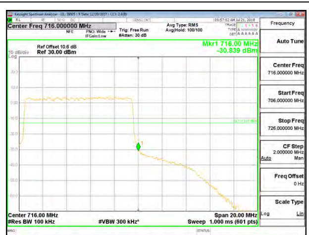
LTE B12 10MHz QPSK High Channel RB50-0
