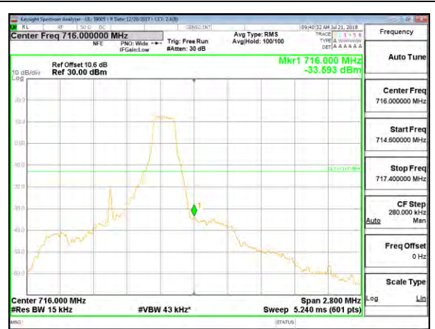
LTE B12 1.4MHz QPSK High Channel RB1-0
