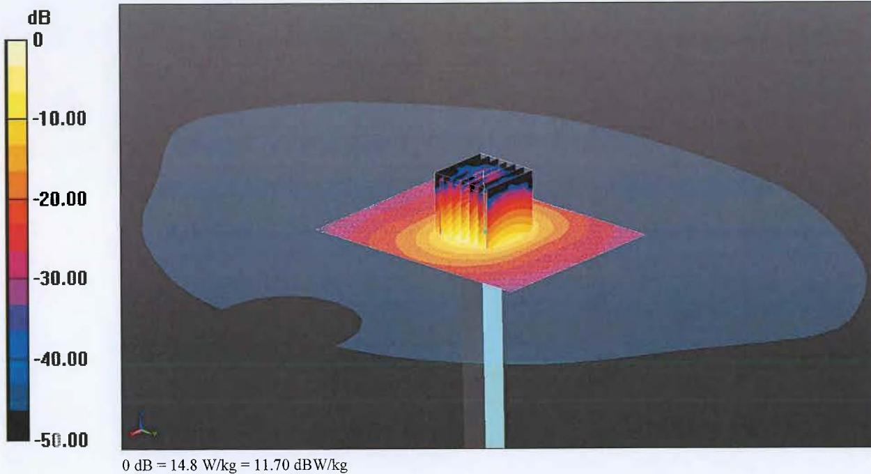
Communication System: UID 0, CW (0); Frequency: 5250 MHz; Duty Cycle: 1:1
