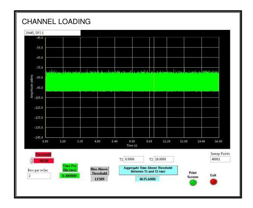
The level of traffic loading on the channel by the EUT is 46.35%.
