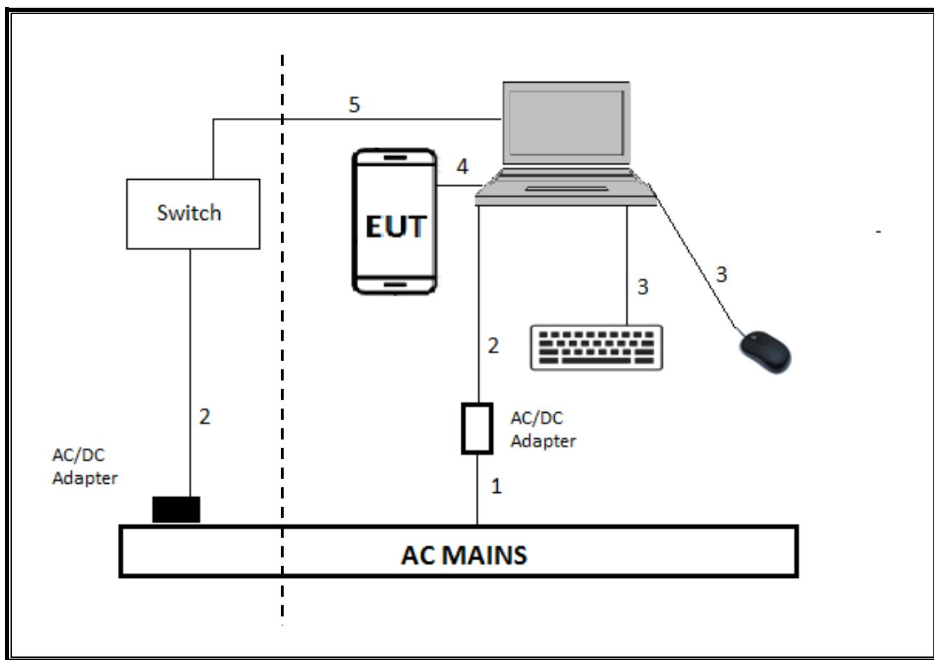
NOTE: Switch location is outside chamber (located in the control room).
