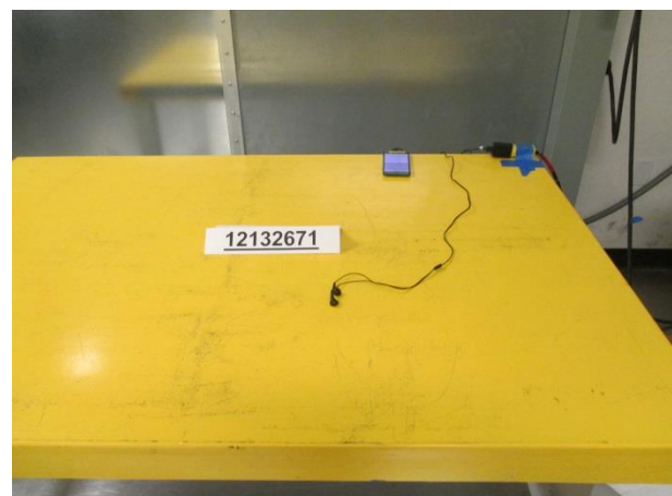
LINE CONDUCTED FRONT PHOTO (CHARGING MODE)
