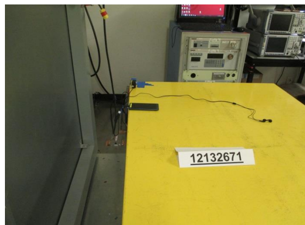
LINE CONDUCTED FRONT PHOTO (CHARGING MODE)
