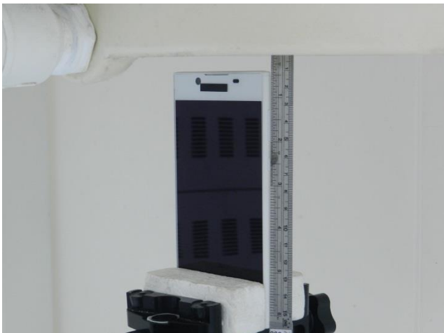
Top Side, Test Separation 10 mm
