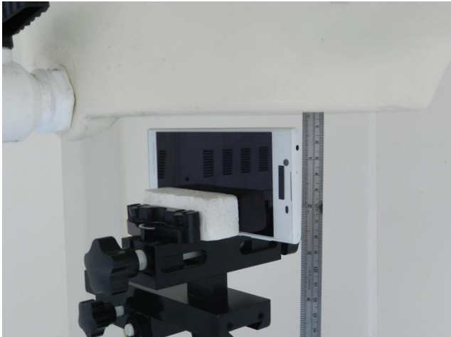
Left Side, Test Separation 10 mm
