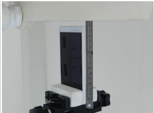
Bottom Side, Test Separation 10 mm
