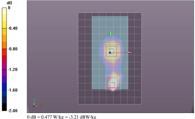
Frequency: 1880 MHz; Duty Cycle: 1:1; Room Ambient Temperature: 24.0°C; Liquid Temperature: 23.0°C Medium parameters used: f = 1880 MHz;  $\sigma$  = 1.359 S/m;  $\epsilon_r$  = 39.739;  $\rho$  = 1000 kg/m<sup>3</sup> DASY5 Configuration:
