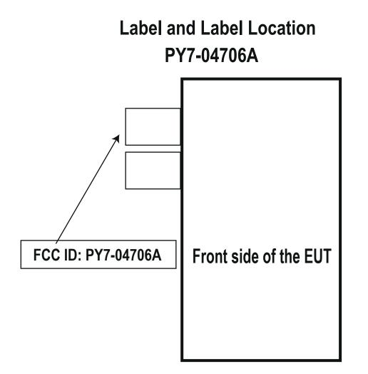
The FCC ID is not on the exterior of the device but labelling meets the conditions allowed in KDB 784748 for the label to be placed in a user accessible area:
