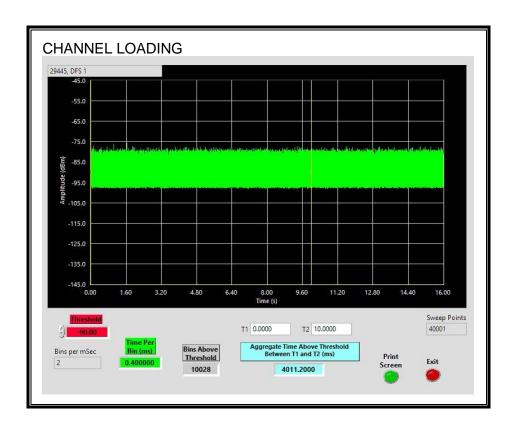
The level of traffic loading on the channel by the EUT is 40.11%.
