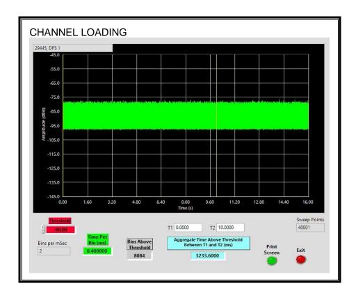
The level of traffic loading on the channel by the EUT is 32.33%.
