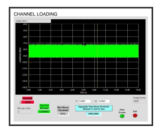
The level of traffic loading on the channel by the EUT is 39.09%.
