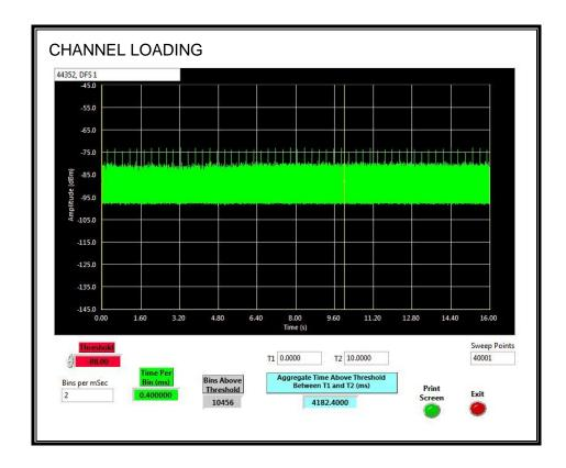
The level of traffic loading on the channel by the EUT is 41.824%.
