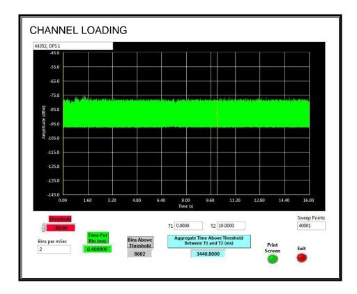
The level of traffic loading on the channel by the EUT is 34.408%.
