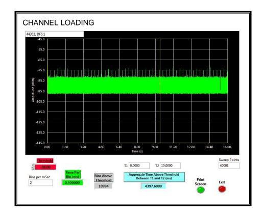
The level of traffic loading on the channel by the EUT is 43.976%.
