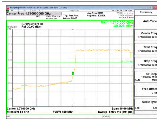
LTE B4 5MHz QPSK Low Channel RB25-0
