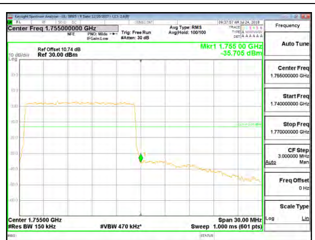
LTE B4 15MHz 16QAM High Channel RB75-0
