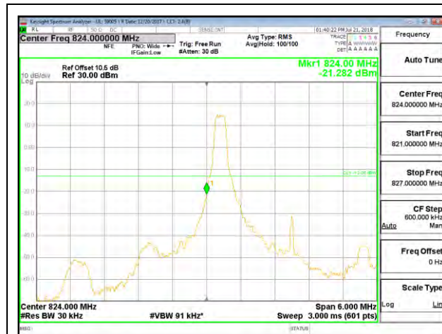
LTE B5 3MHz QPSK Low Channel RB1-0
