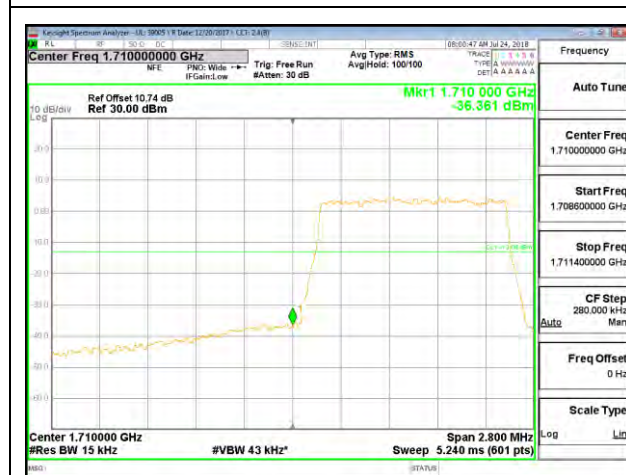
LTE B4 1.4MHz 16QAM Low Channel RB6-0
