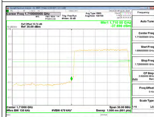
LTE B4 15MHz 16QAM Low Channel RB75-0
