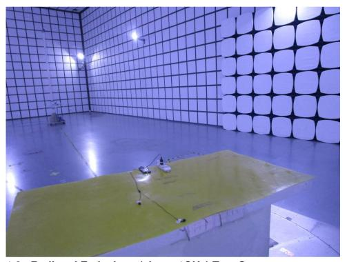
1.3 Radiated Emissions (above 1GHz) Test Setup
