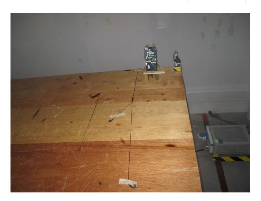
1.2 Radiated Emissions(30MHz-1GHz) Test Setup
