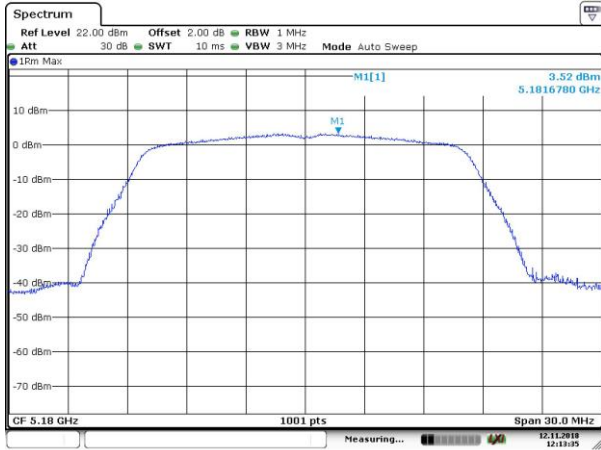
802.11a 5150~5250 MHz Power Spectral Density Data Plot (CH Low 5180 MHz)
