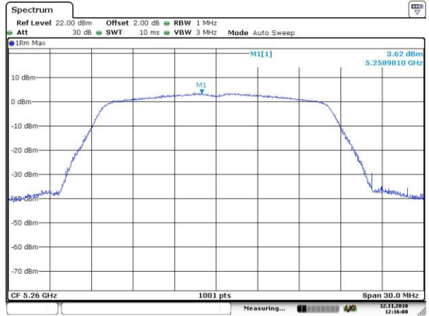
802.11a 5250~5350 MHz Power Spectral Density Data Plot (CH Low 5260 MHz)
