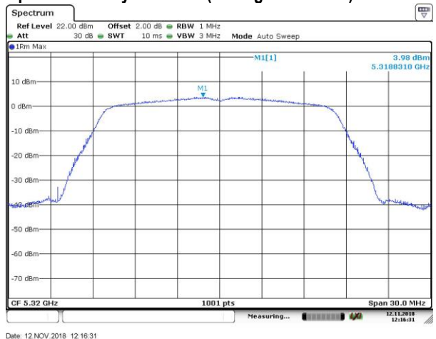
Power Spectral Density Data Plot (CH High 5320 MHz)
