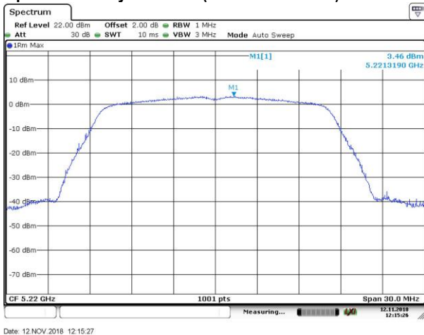
Power Spectral Density Data Plot (CH High 5240 MHz)
