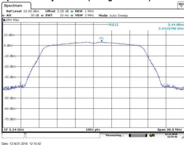
Power Spectral Density Data Plot (CH High 5240 MHz)
