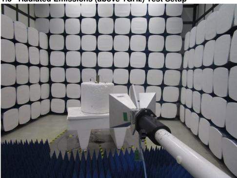
1.3 Radiated Emissions (above 1GHz) Test Setup
