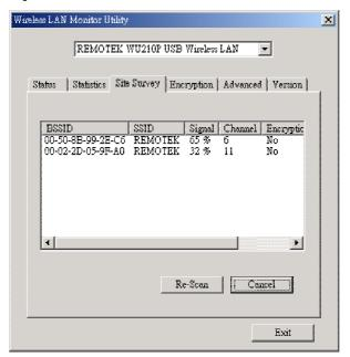
It shows all APs or adaptors in Ad-Hoc mode nearby. You may click **Re-Scan** to collect the wireless device information to know the BSSID and Ch(Channel). If you want to connect to any device on the list, double-click on the device. The adaptor will connect to the device you have selected.
