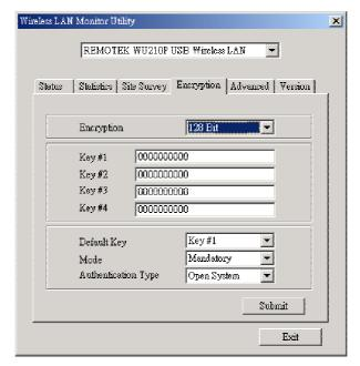
You may desire an additional measure of security on your wireless network, which can be achieved by using WEP(Wired Equivalent Privacy) encryption. WEP encrypts each frame transmitted from the radio using one of the keys entered from this panel. When an encrypted frame is received it will only be accepted if it decrypts correctly. This will only happen if the receiver has the WEP key used by the transmitter.
