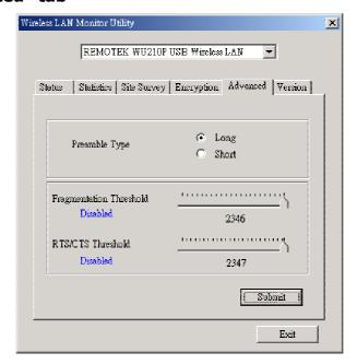
We can find and change some advance settings here. They are **Preamble Type, Fragmentation Threshold**, and **RTS/CTS Threshold**. Note that the adaptor has a feature to select the preamble type from AP automatically.
