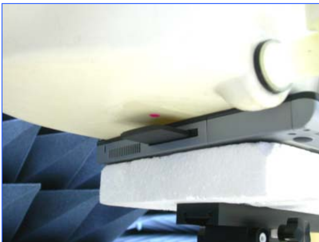
Figure 13. Top (Notebook PC touching SAM Phantom) Distance of the PCMCIA card to the phantom = 1.0 cm The laptop computer was opened in this position.
