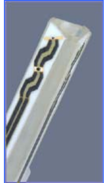
Figure 4. ET3DV6 E-field Probe
