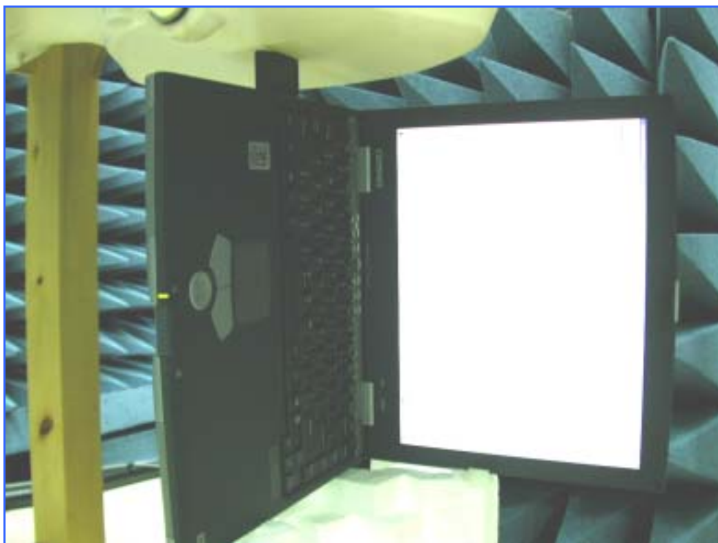
Figure 12. Left side (PCMCIA card touching SAM Phantom) Distance of the PCMCIA card to the phantom = 0 cm
