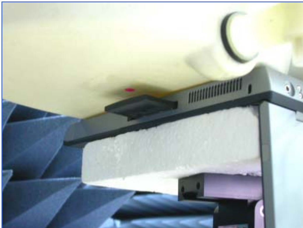
Figure 11. Bottom (Notebook PC touching SAM phantom) Distance of the PCMCIA card to the phantom = 1.0 cm
