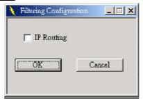
If you check IP Routing, only IP Packets will pass through AP between Ethernet and Wireless LAN.
