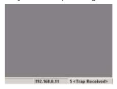
When AP SNMP Manager receives trap messages from AP, " # < Trap Received > " will appear on bottom-right of AP SNMP Manager.
