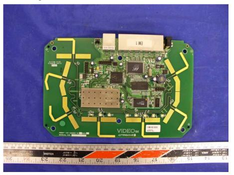
Board – Top View without Shielding
