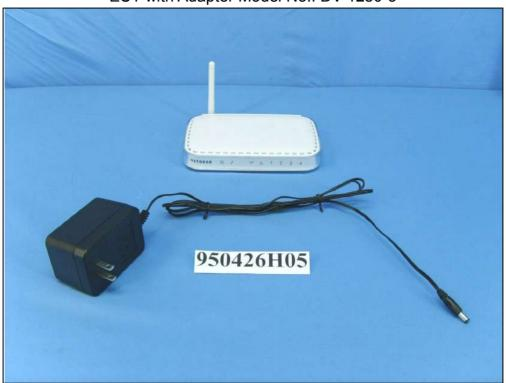
EUT with Adapter Model No.: DSA-0131F-12
