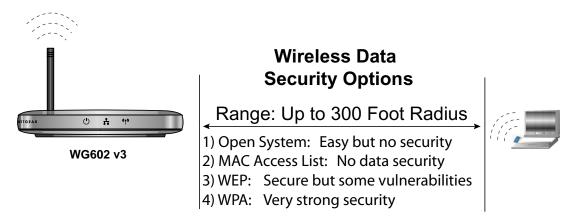
Figure 3-1: WG602 v3 wireless data security options
