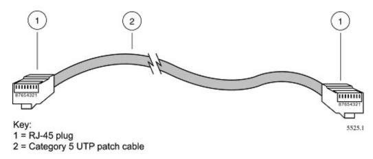
Figure C-3: Category 5 UTP Cable with Male RJ-45 Plug at Each End
