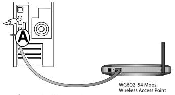
Figure 3-2: Set up the WG602 v3
