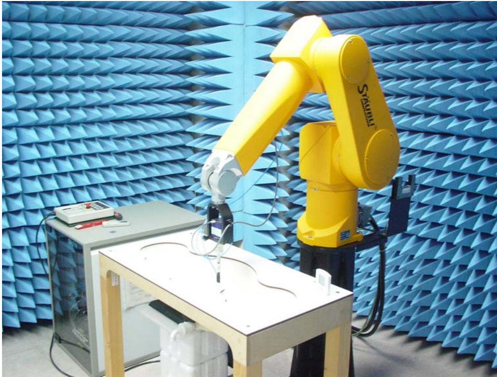
Fig.1 Photograph of the SAR measurement System
