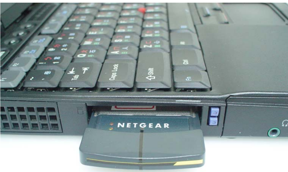
Fig.11 With IBM ThinkPad T30 PCMCIA slot
