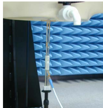
Photograph of the 2450MHz System Check
