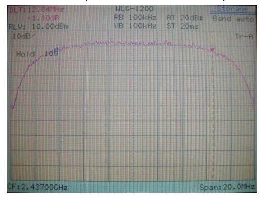
802.11g Channel 6: 16.80MHz (The minimum 6dB BW at least 500kHz)
