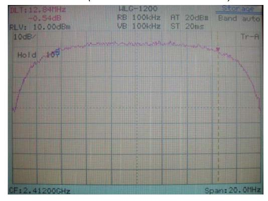
802.11g Channel 1: 16.80MHz (The minimum 6dB BW at least 500kHz)
