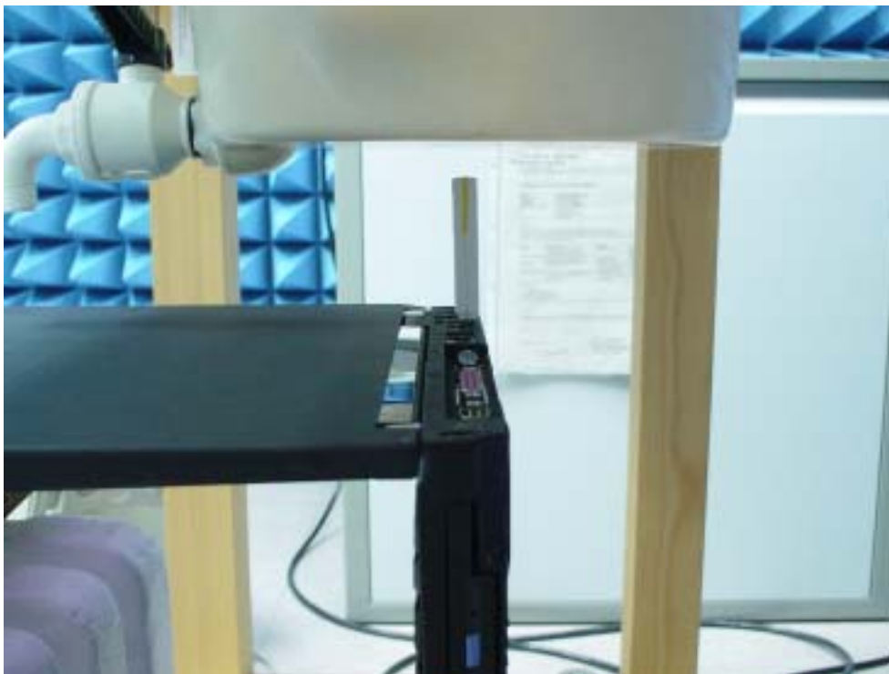
Fig.4 Photograph of the antenna tip is upward and at a distance of 1.5 cm from the base of the phantom.
