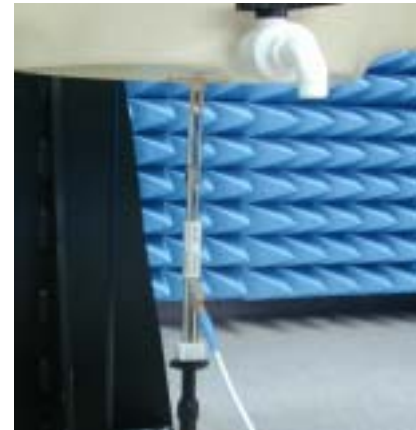
Photograph of the 2450MHz System Check
