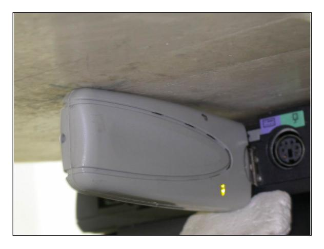
The lateral side of the EUT to the flat phantom distance 0mm
