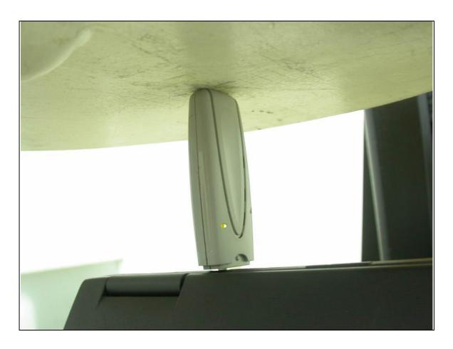
The tip of the EUT to the flat phantom distance 0mm
