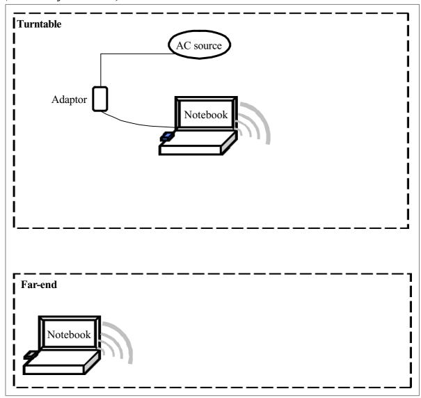
The tests below are carried out the EUT transmitter set at high power in TDD mode. The EUT is needed to force selection of output power level and channel number.
