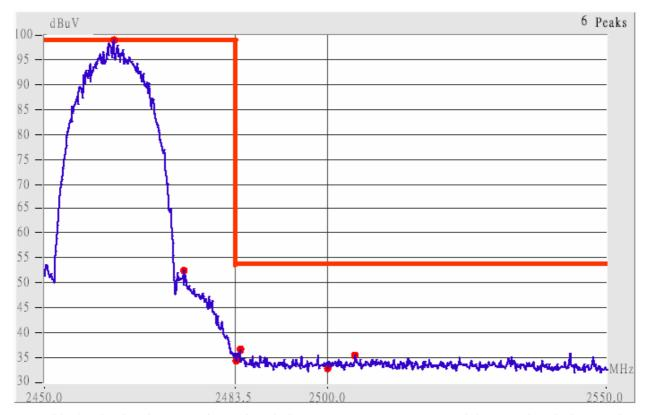
This is the hard copy of our bandedge measurement generated by our bandedge testing program. The plot shown above is the bandedge of channel 11.
