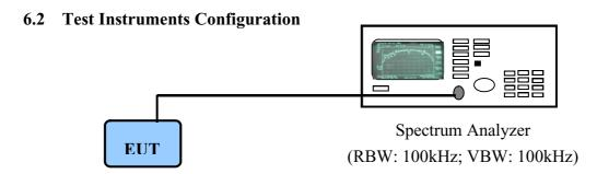
P.S.: Notebook computer to control the EUT at maximal power output and channel Number and set antenna kit
