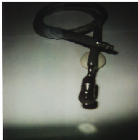
Fig. d. Photograph of the Hewlett Packard Model 85070B Dielectric Probe. This is an open-circuited coaxial line probe.
