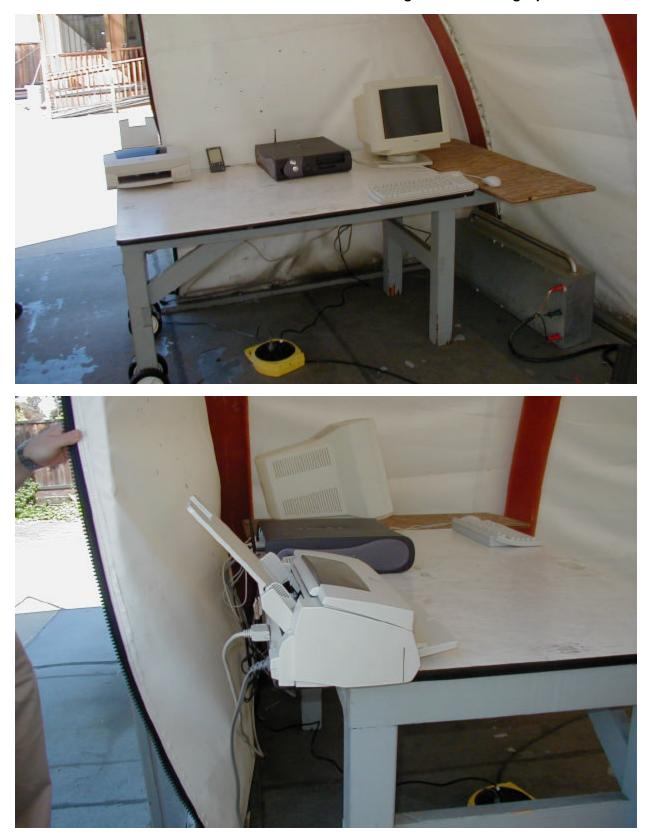
AC Power Line Conducted Emissions Test Configuration Photographs
