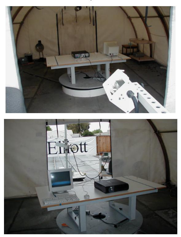
Radiated Emissions – Radio Spurious Emissions Above 1GHz
