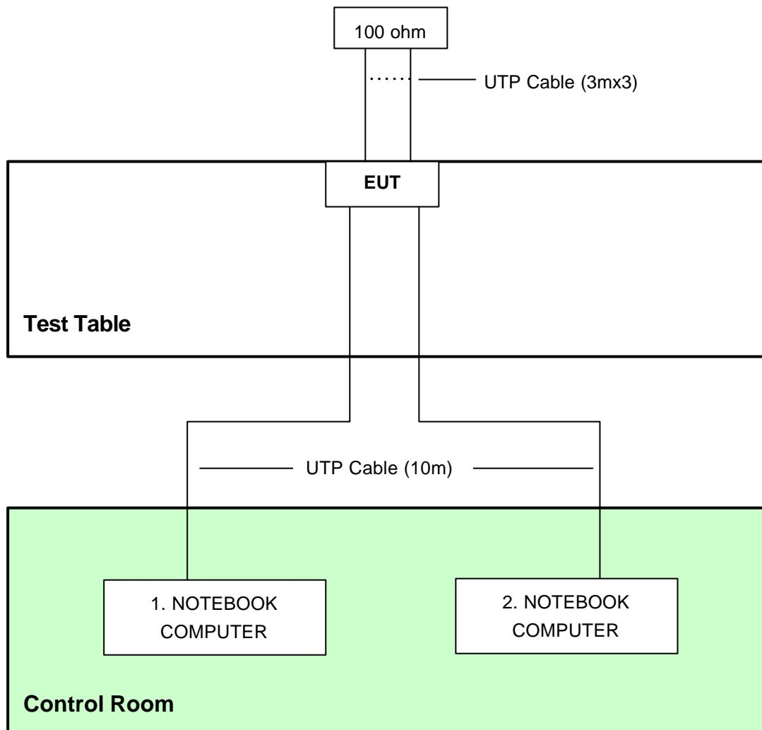
**NOTE:** 1. Support units 1-2 were kept in the control room during the test.
