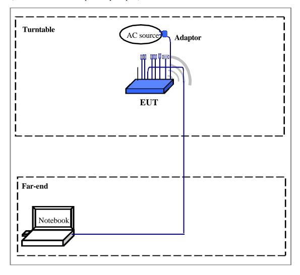
The tests below are carried with the EUT transmitter set at high power in TDD mode. The EUT is forced to select of output power level and channel number by notebook computer.
