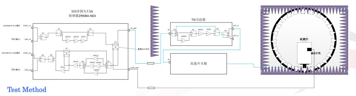
The "great circle" cut method, whereby the Measurement Antenna remains fixed and the EUT is rotated about two axes in sequential order. The radiated RF performance of the Equipment Under Test (EUT) is measured by sampling the radiated transmit power of the mobile at various locations surrounding the device. A three-dimensional characterization of the 'transmit' performance of the EUT is pieced together by analyzing the data from the spatially distributed measurements.
