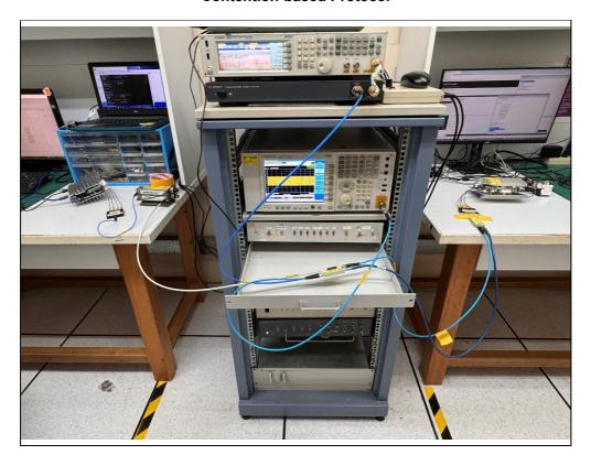
Multi-Antenna Systems Directional Gain measurement
