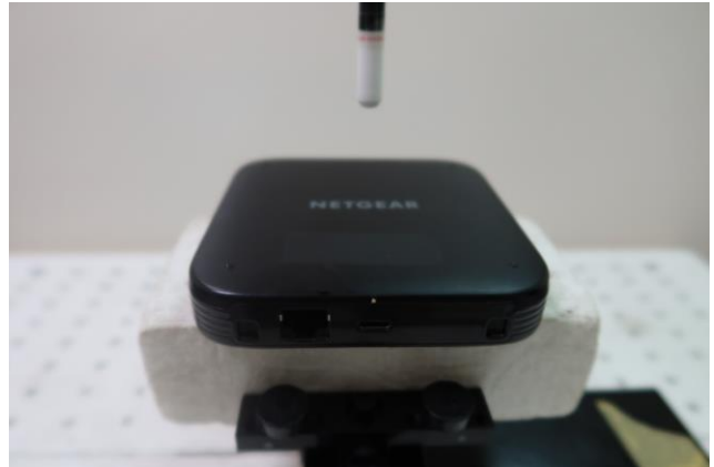
Bottom, Test Separation 10 mm
