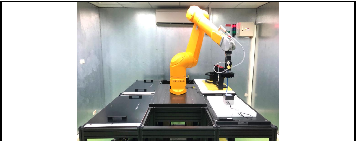
Fig-3.2 SPEAG DASY6 System
