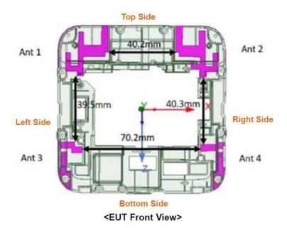
The separation distance for antenna to edge:
