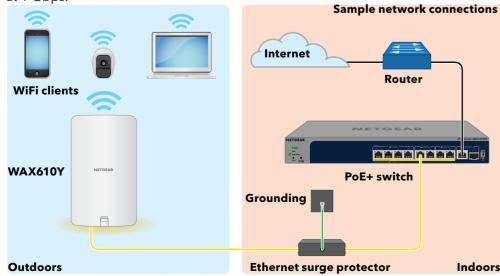
The access point receives an IP address from a DHCP server (or a router that functions as a DHCP server) in your network. If your network does not include a DHCP server, the access point uses its default IP address 192.168.0.100.
