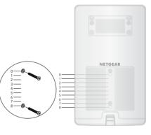
2. Drill holes into the wall for the two anchors in which you will insert the screws.
