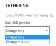
Your settings are saved. When you connect the USB type C cable, the mobile router battery charges, but you cannot use the tethered connection to access the mobile hotspot with a web browser.
