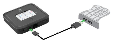
The Battery icon on the LCD indicates that the battery is charging.
