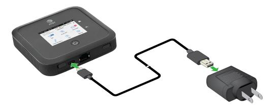
Plug the wall charger into a wall socket.The Battery icon on the LCD indicates that the battery is charging.
