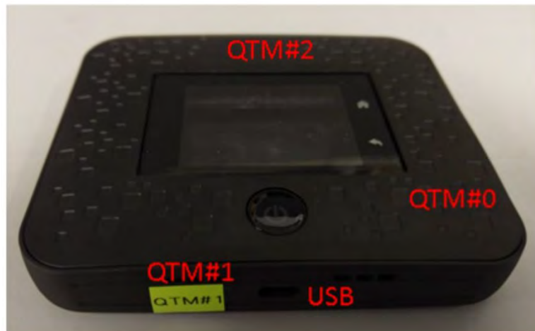
Figure 3-1: Netgear 5G MHS Travel Router (FCC ID: PY319100441) with three QTM052 mmW antenna modules
