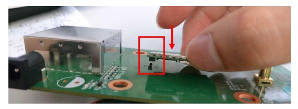
Caution: An inappropriate installation will break the board to board connectors permanently.
