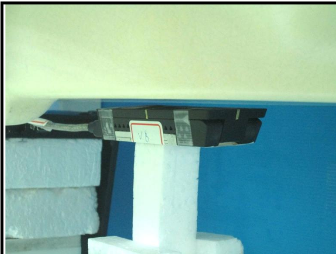
USB Horizontal Down with ANT at 0 Degree Test at 5 mm Separation Distance
