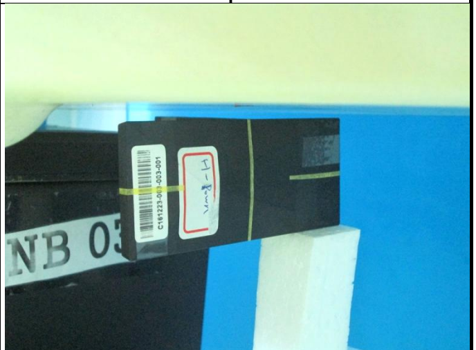
USB Vertical Front with ANT at 90 Degree Test at 5 mm Separation Distance
