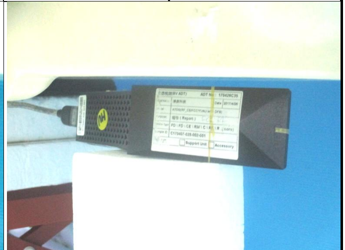
USB Vertical Back with ANT at 160 Degree Test at 5 mm Separation Distance
