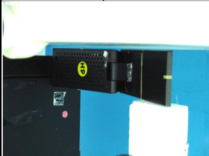
USB Vertical Front with ANT at 160 Degree Test at 5 mm Separation Distance
