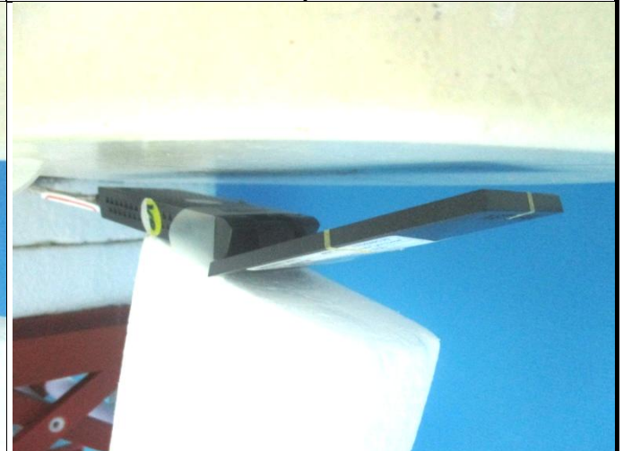
USB Horizontal Down with ANT at 160 Degree Test at 5 mm Separation Distance
