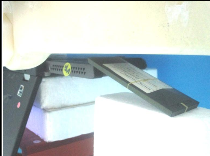
USB Horizontal Up with ANT at 160 Degree Test at 5 mm Separation Distance
