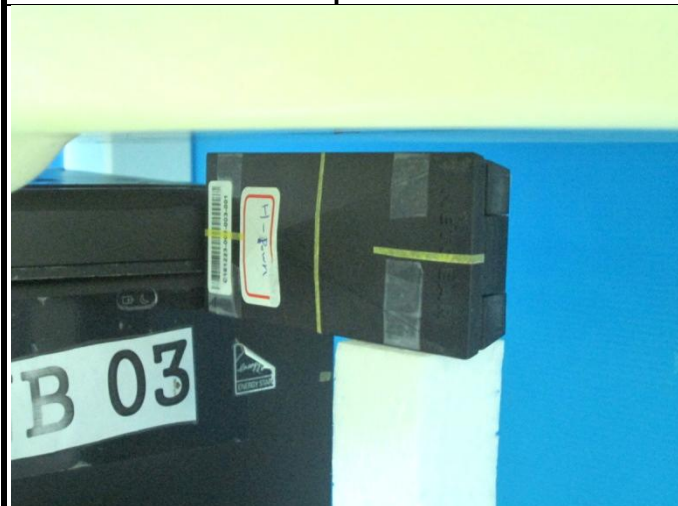
USB Vertical Front with ANT at 0 Degree Test at 5 mm Separation Distance
