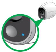
After the camera syncs, the Power LED on the base station might start blinking. This indicates that the camera's firmware is updating. For information about firmware updates, see *Arlo Camera Firmware Updates* on page 11.
