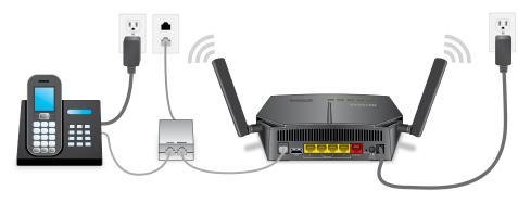
Connect the DSL port on the modem router to a DSL outlet.
