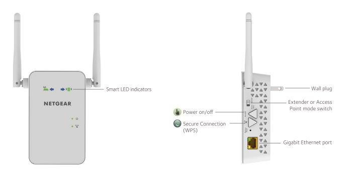
Smart LED indicators help find the best extender placement for optimal WiFi coverage while displaying real-time, extender network status.
