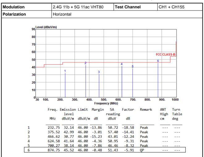
Note 1: Emission Level (dBuV/m) = SA Reading (dBuV/m) + Factor\* (dB)
